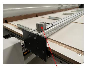
**The back fence** includes pneumatic clamping devices. It is lowerable so to disappear under the working surface when it is not used.
