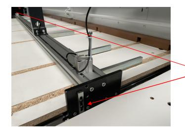
Two slide ways with accurate linear ball-bearings
