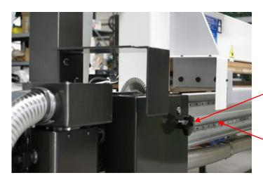
Handwheel for the adjustment of the saw blade axial positon. Stepless adjustment range  $0 \div 3$  mm
